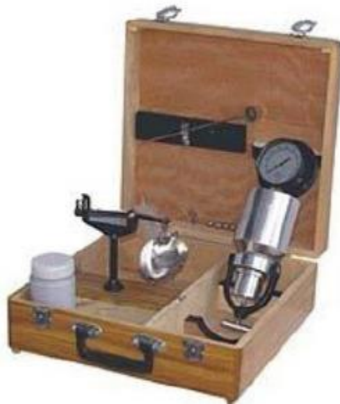
Setup for Rapid Moisture content Determination
